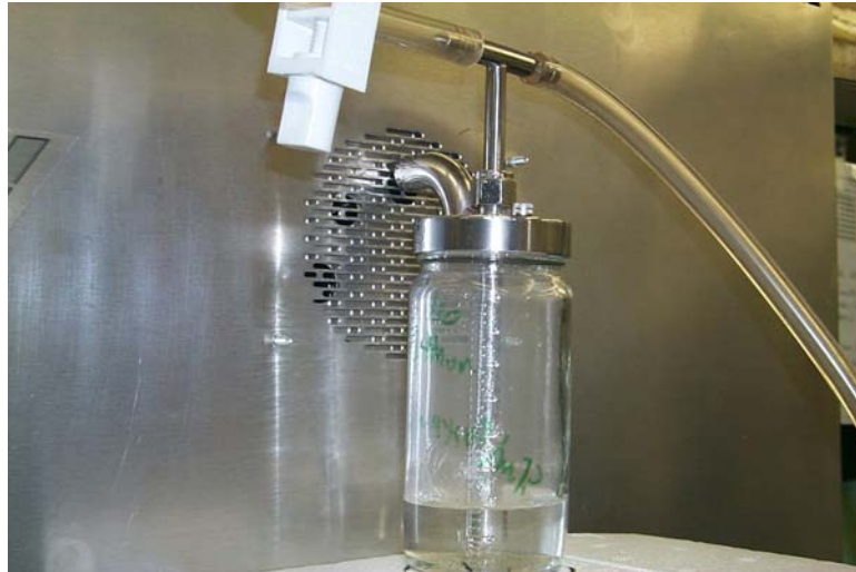
Figure 2 – Suspension of B. thuringiensis spores in nebulizer and introduced into the AiroCide.
