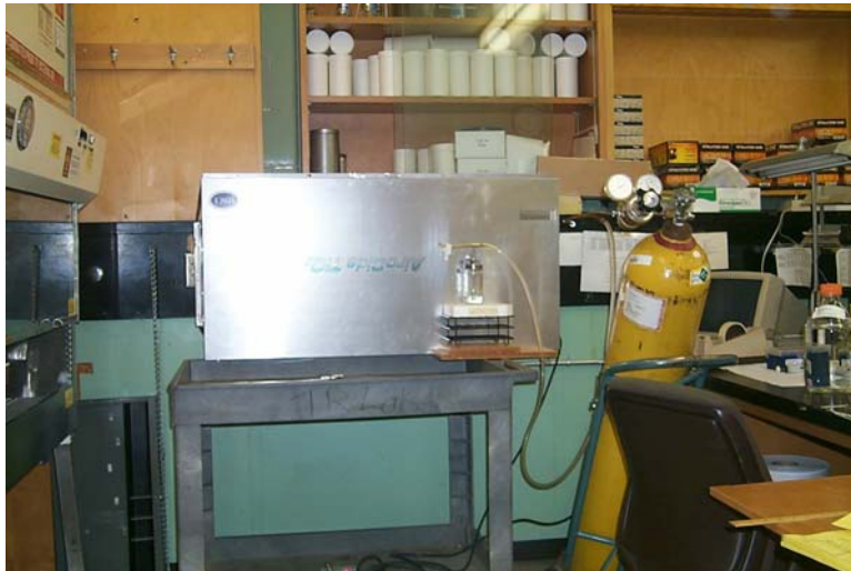
Figure 3 – Experimental set-up. Air from a cylinder aerosolizes suspension of B. thuringiensis spores.
